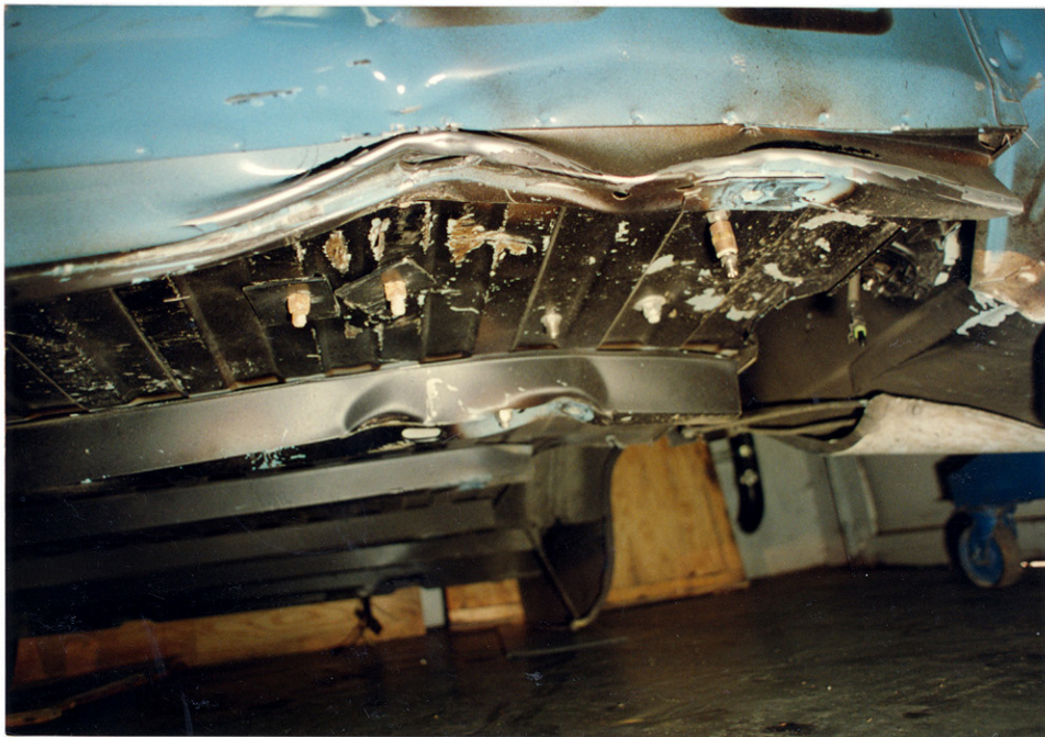
32. Damage to the Floor and Crossmembers of the Cargo Box of the Pickup Truck
